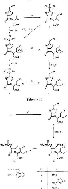
$H_2SO_4$ -CHCl<sub>3</sub> system gave trichloride 2 in 80% yield after passage of 15 F/mol of electricity. Without isolation, continued electrolysis under irradiation with a 750-W halogen lamp afforded pentachloride 3 in 50% overall yield after an additional 5 F/mol of electricity was passed. The successful conversion of 2 to 3 was achieved by treatment with chlorine in  $CH_2Cl_2$  under illumination for 10 min (90% yield).
